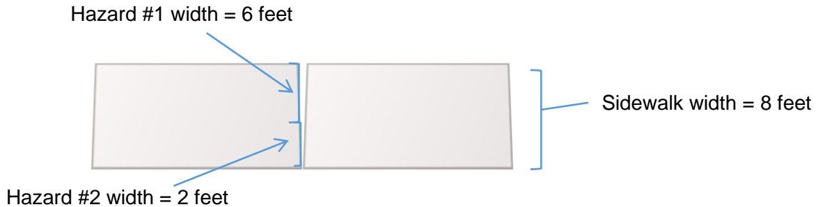
Figure 1: Panels Over 6 Feet Wide
